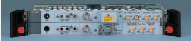
MU150121A 10/10.7G Optical Unit (Tx)
